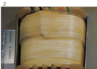
1_ASR Emitter separate power supply 2_Philbert-Mantelschnitt-transformer
